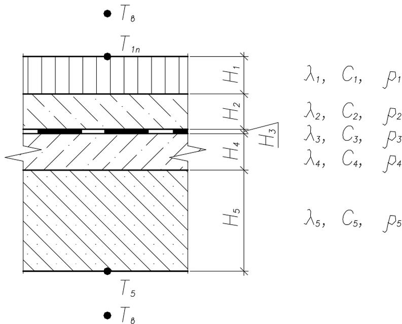
**Fig. 2.** Design scheme of a road bridge floor for calculating the temperature conditions
