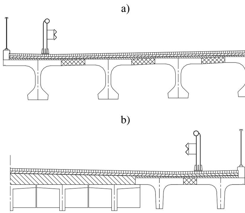
**Fig. 1.** Types of bridge cross-section:
