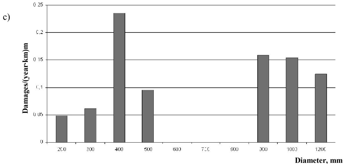
**Fig. 3 (end).** Damage distribution of main heat supply networks by PC Saratov heat supply network in pipeline inner diameters: c) 2008
