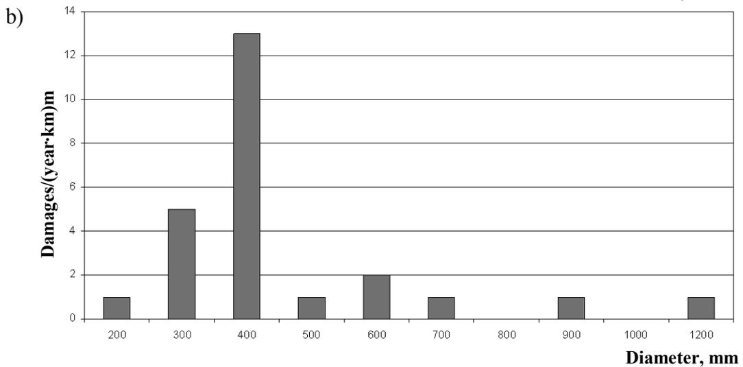
**Fig. 2.** Damage distribution of main heat supply networks
