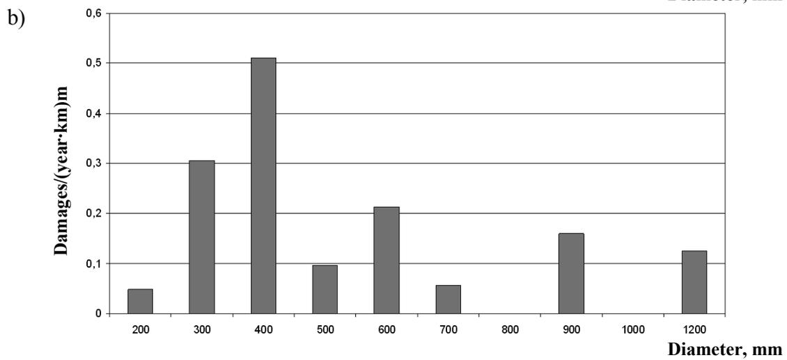
**Fig. 3.** Damage distribution of main heat supply networks by PC Saratov heat supply network in pipeline inner diameters: a) 2006; b) 2007
