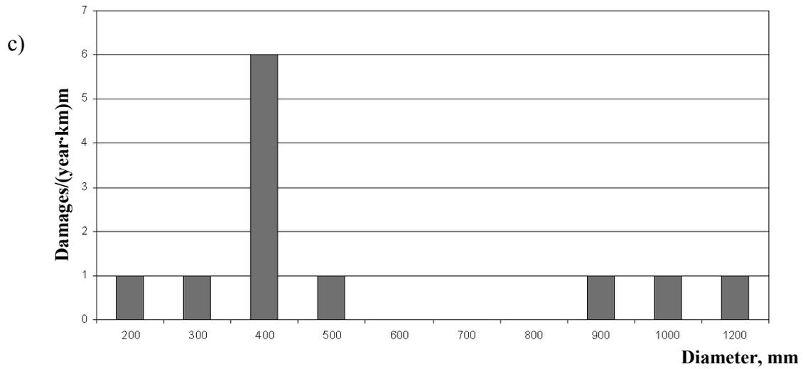
**Fig. 2 (end).** Damage distribution of main heat supply networks by PC Saratov heat supply network in pipeline inner diameters: c) 2008
