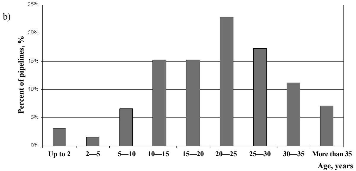
**Fig. 1b.** Length and age group of main heat supply networks by PC Saratov
