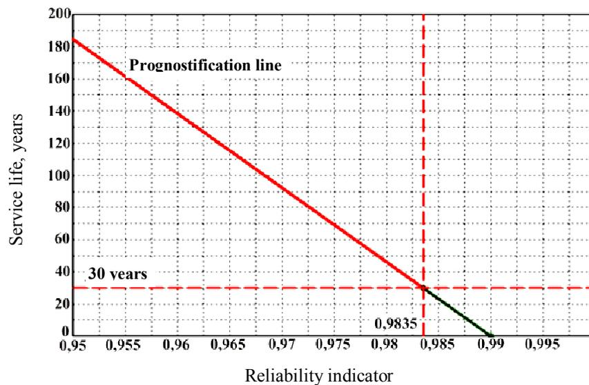
**Fig. 2.** Evaluation of a residual service life using the reliability indicator
