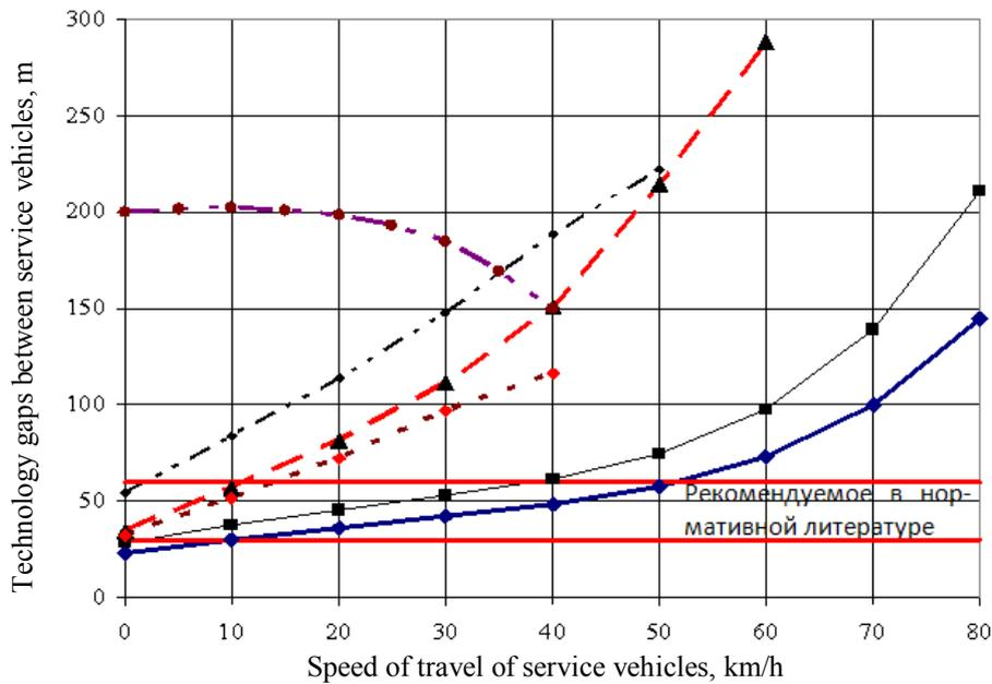
**Fig. 4.** Technology gaps between road service vehicles ensuring a safe overtaking: рекомендуемое в нормативной литературе — as set out in the guidance literature;
