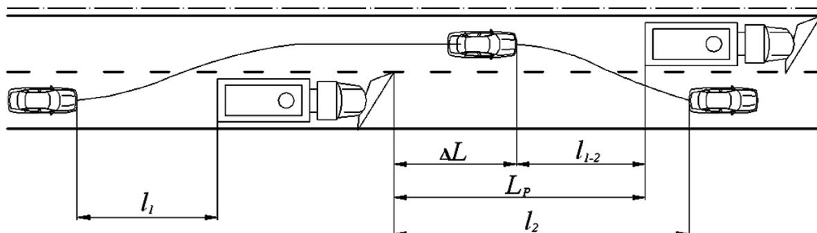
**Fig. 2.** Calculation scheme of overtaking during the operation of the maintenance fleet
