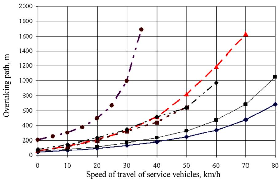
Fig. 3. Safe overtaking distance for different states of road surfaces:
