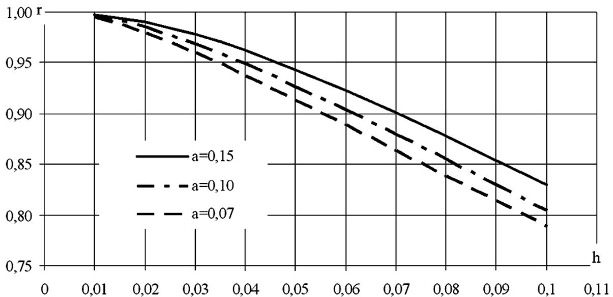
Fig. 5. Dependency of the coefficient of thermal and engineering integral  $r$  on the height of the rib  $h$
