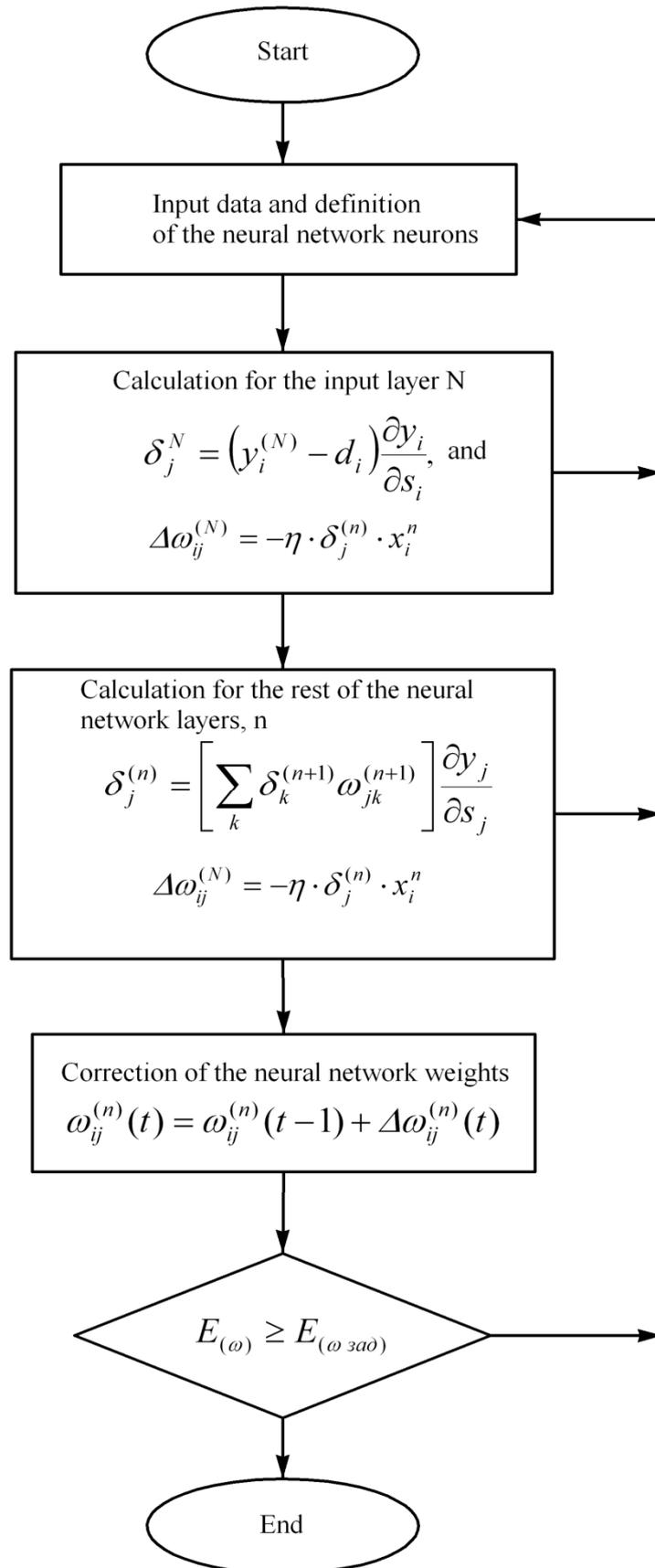
Fig. 3. Learning algorithm for the developed artificial neural network
