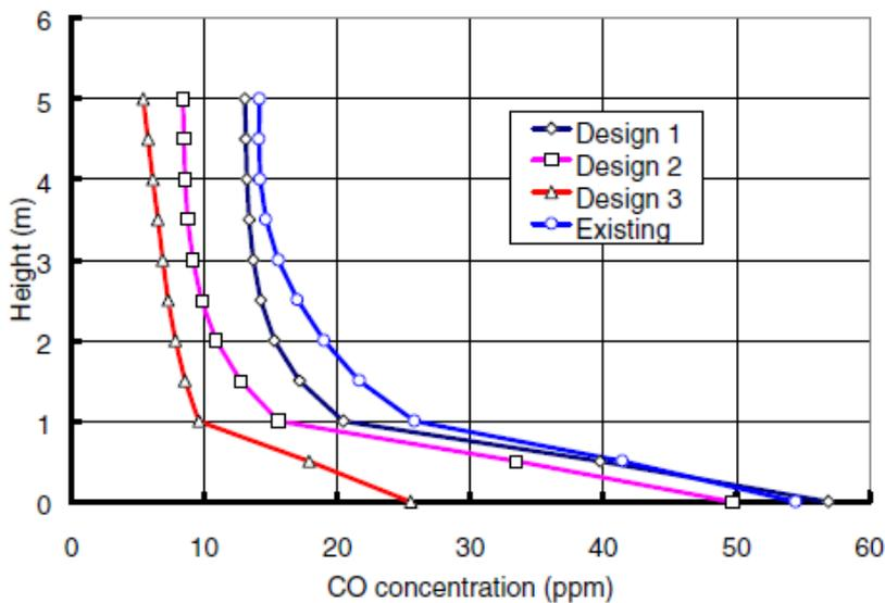
**Fig. 5.** Distribution of CO over the ice surface in different air distribution schemes
