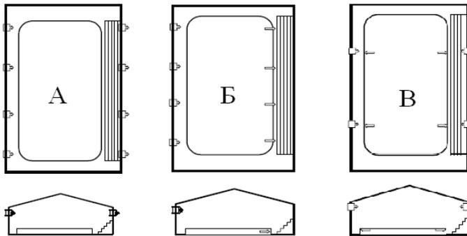
**Fig. 4.** Schematic of air exchange in covered ice rinks
