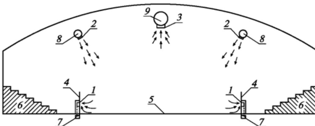
**Fig. 3.** Organization of distribution of air according to the mixed scheme:
