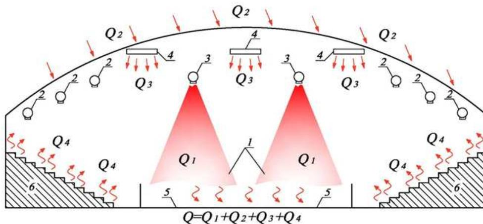
**Fig. 1.** Schematic diagram of impact of the perceived heat inflows on the surface of ice:
