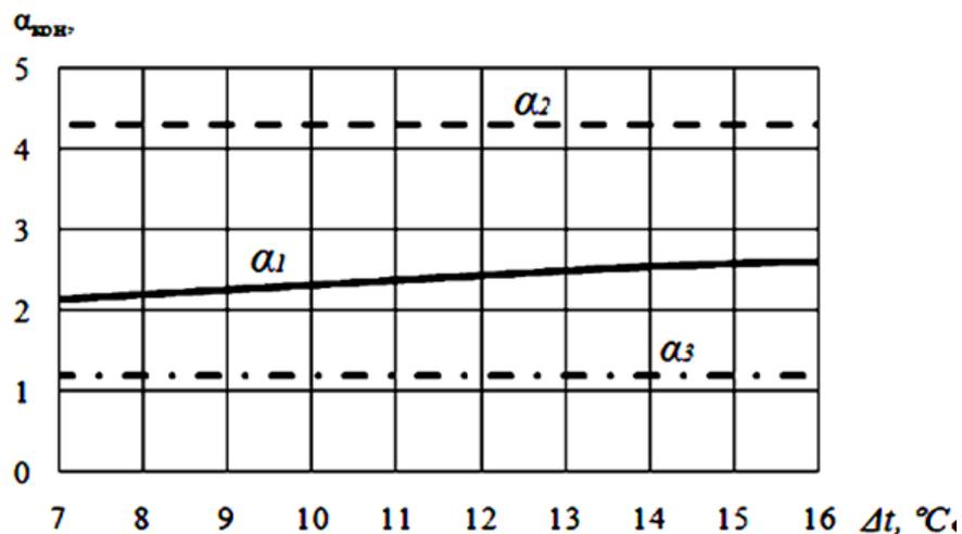
**Fig. 2.** The dependence of the heat return coefficient at convective heat exchange on the difference in temperatures  $\Delta t$ :  $\alpha_1$ ,  $\alpha_2$  and  $\alpha_3$  — heat return coefficients are calculated according to formulas (5), (6) and (7), respectively
