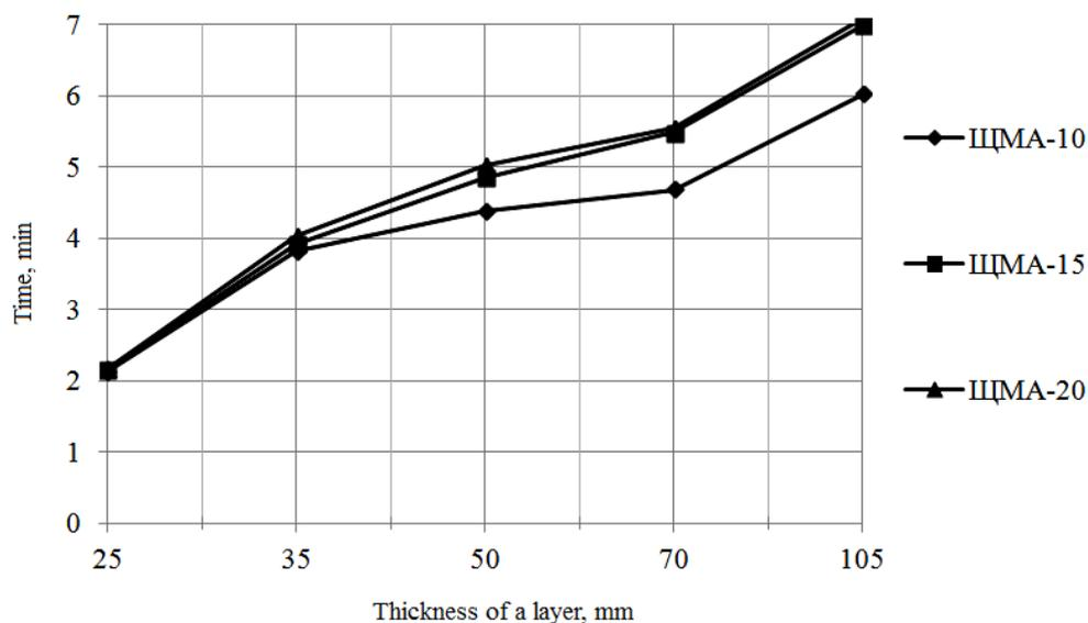
**Fig. 5.** Dependence of the strength increase (stone-asphalt concrete mix -10, stone-asphalt concrete mix -15, stone-asphalt concrete mix -20) on the relative thickness of the layer (temperature — 80 °C)
