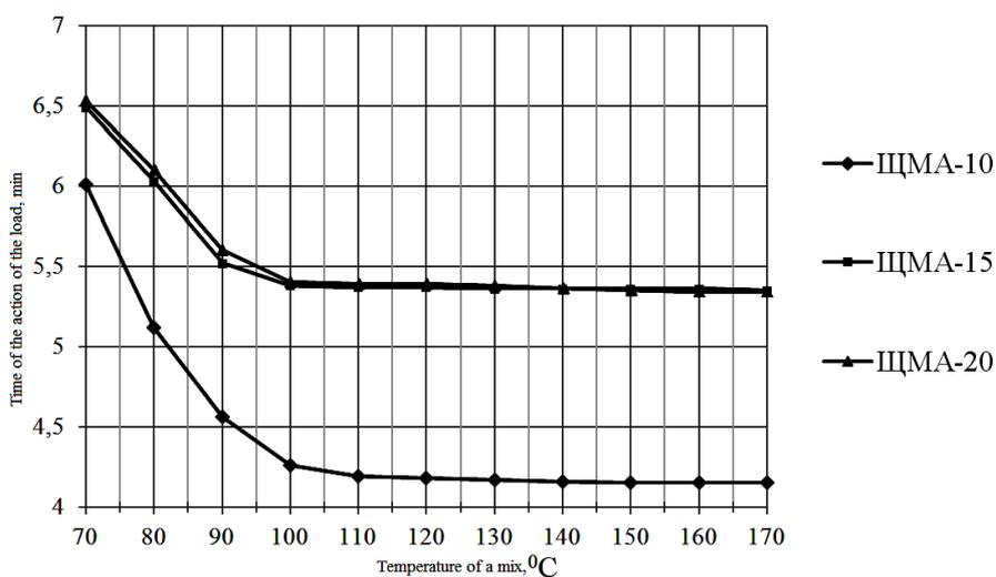
**Fig. 1.** Load-temperature dependence to achieve the required strength of asphalt concrete: stone-asphalt concrete mix -10, stone-asphalt concrete mix -15, stone-asphalt concrete mix -20,  $h = 70$  mm,  $D = 70$  mm,  $P = 40$  MPa,  $S = 3$  mm/min, БНД bitumen 60/90
