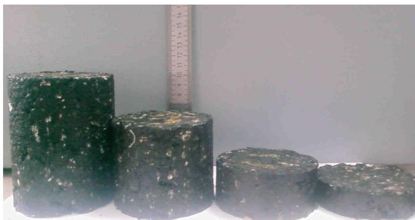
**Fig. 2.** Stone-asphalt concrete mix samples for defining the effect of the thickness of a road surface layer on the strength parameters
