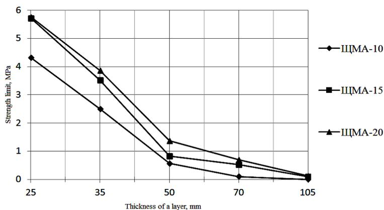
**Fig. 3.** Dependence of the compression strength (stone-asphalt concrete mix -10, stone-asphalt concrete mix -15, stone-asphalt concrete mix -20) on the relative thickness of a layer (temperature — 80 °C)
