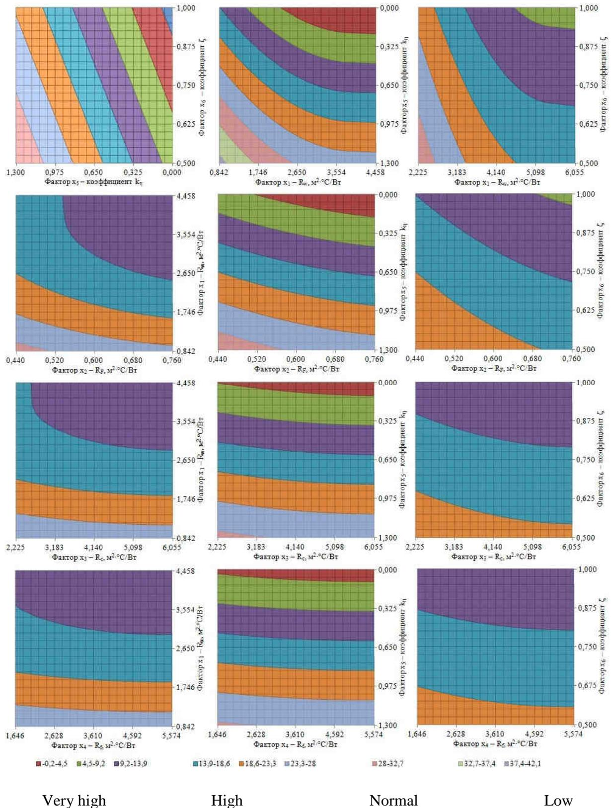
**Fig. 1.** Specific heat energy consumption for the heating of the existing building  $q_h^{des}$ ,  $kJ/(m^3 \cdot ^\circ C \cdot day)$  depending on the combination of different factors (where фактор means factor, коэффициент means coefficient)
