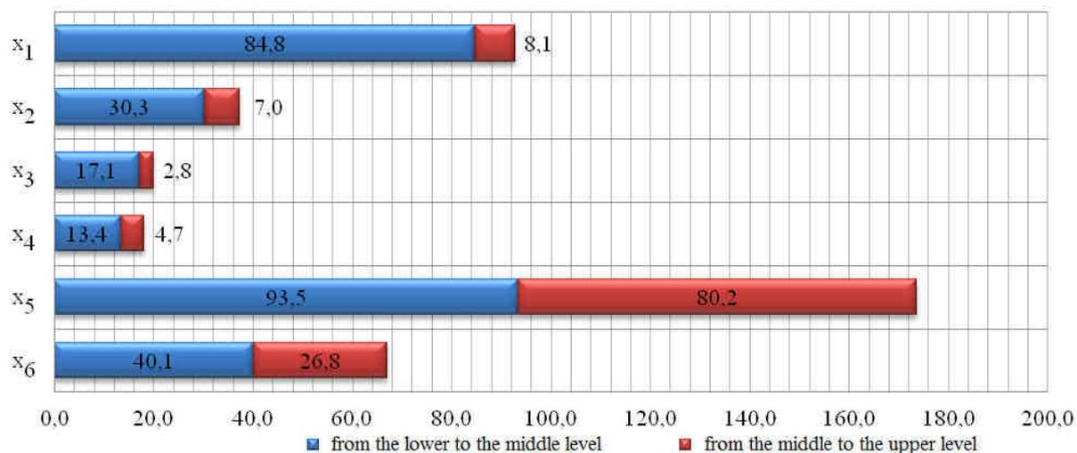
**Fig. 2.** Effect of the examined factors, %, on the specific heat energy consumption on the heating of the existing building  $q_h^{des}$ ,  $\text{kJ}/(\text{m}^3 \cdot ^\circ\text{C} \cdot \text{day})$
