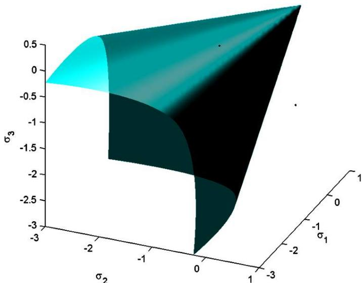
**Fig. 2.** Specific surface in the principal stresses according to the *Willam-Warnke* yield criterion
