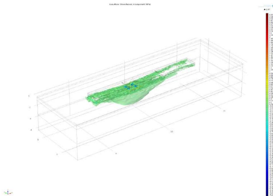
**Fig. 6.** Isofields of normal stresses  $\sigma_z$  in the construction layer of a multi-layer airfield pavement
