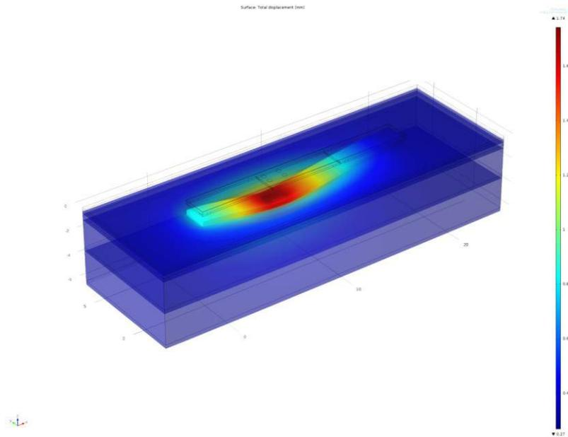
**Fig. 5.** Total deformations of a multi-layer airfield pavement
