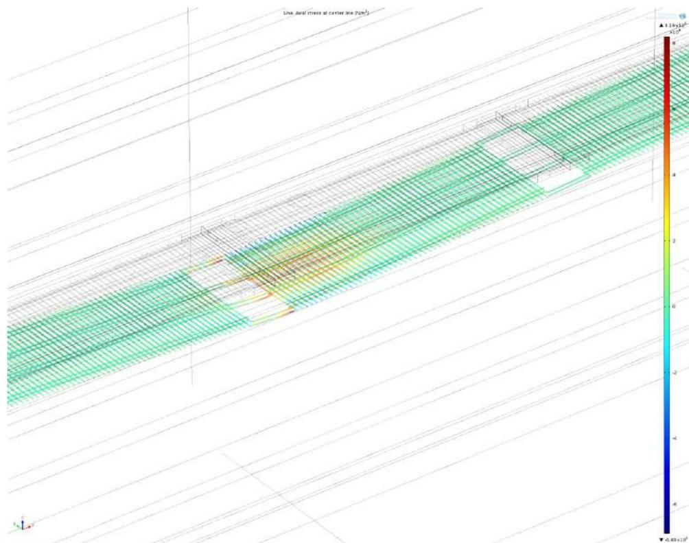
**Fig. 8.** Stresses in the reinforcement carcass of previously stressed ferroconcrete airfield paving ПАГ-14V
