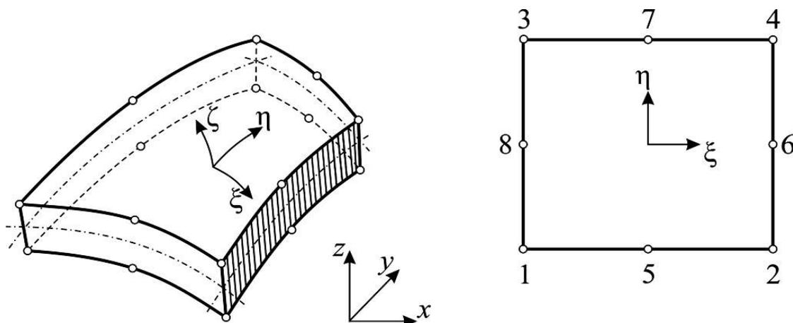
**Fig. 4.** Finite element in the shape of a curvilinear parallelepiped in a local normalized coordinate system  $(\xi, \eta, \zeta)$
