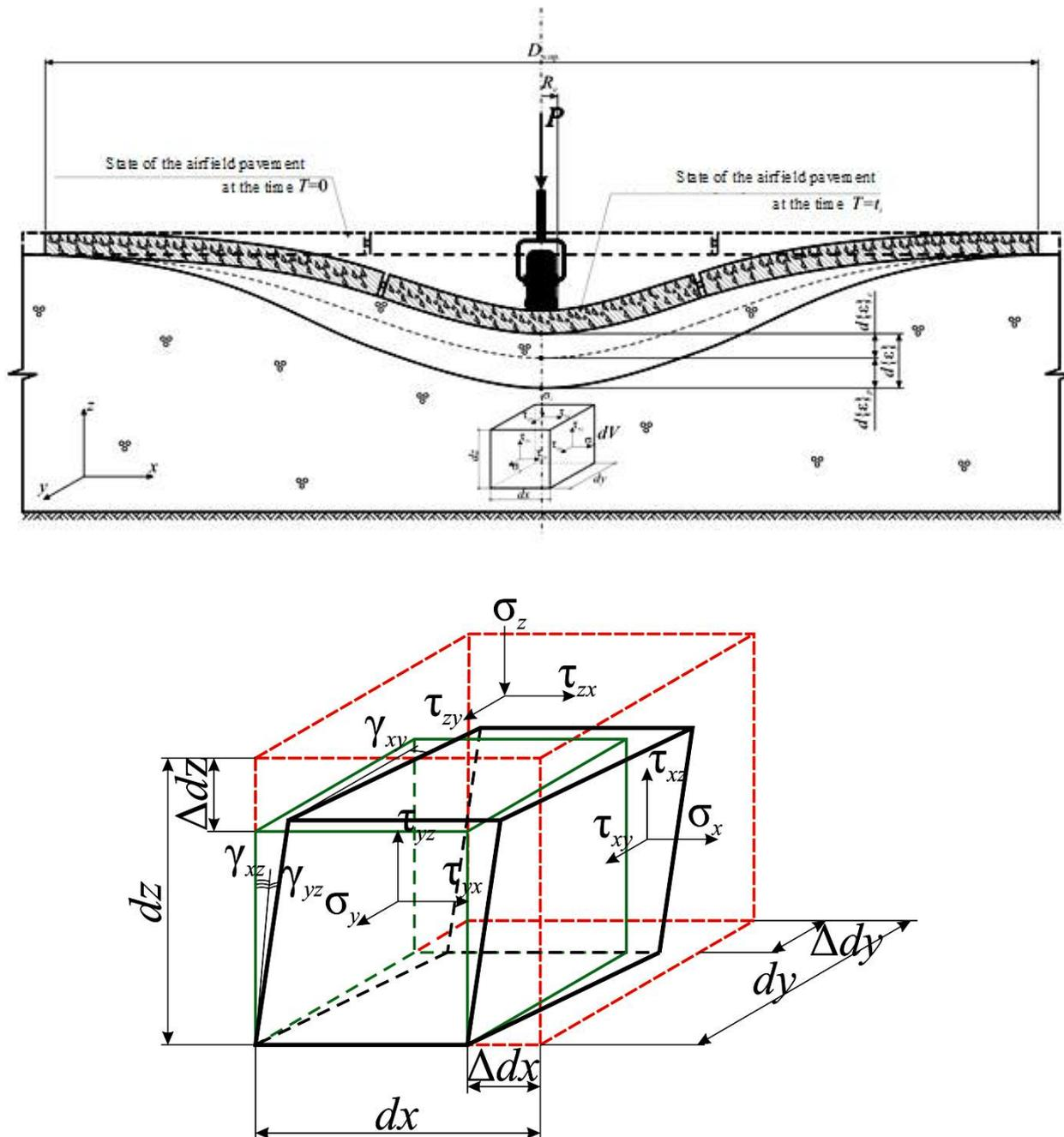
**Fig. 1.** Schematic of a multi-layer airfield pavement under an aircraft wheel load:
