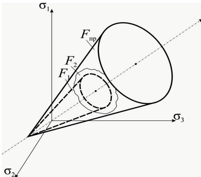
**Fig. 3.** Yield surfaces *Drucker-Prager*:  $F_{np}$  is a specific surface
