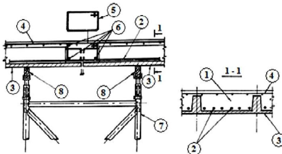
**Fig. 3.** Support scheme for the panels of precast concrete formwork in the middle of the span. A part of the monolithic formwork and reinforcement example (see Fig. 2 for the position of the grid):
