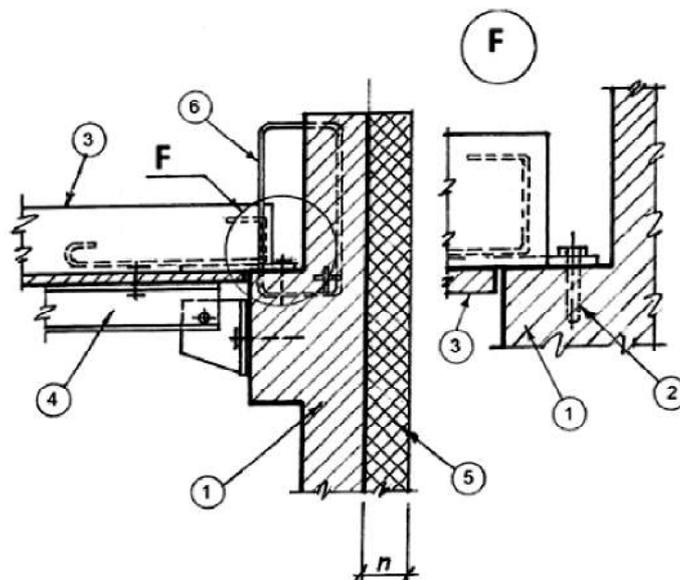
**Fig. 6.** Support scheme of the panels of prefabricated precast concrete formwork on the external wall panel:
