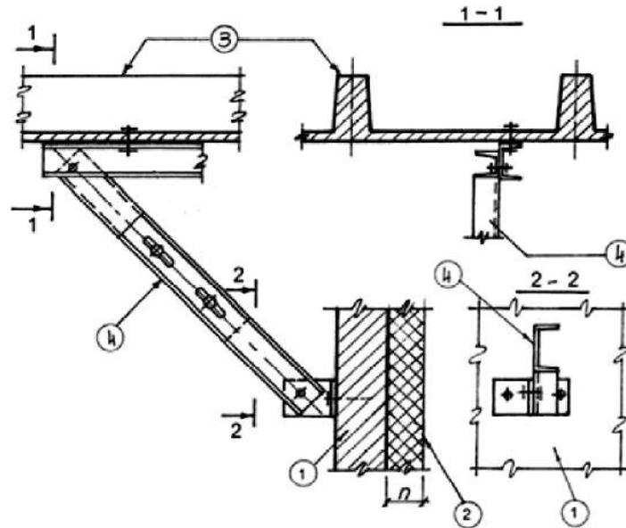
**Fig. 5.** Scheme for fixing a prefabricated precast concrete panel (3) horizontally (see Fig. 2 for the position of the grid):
