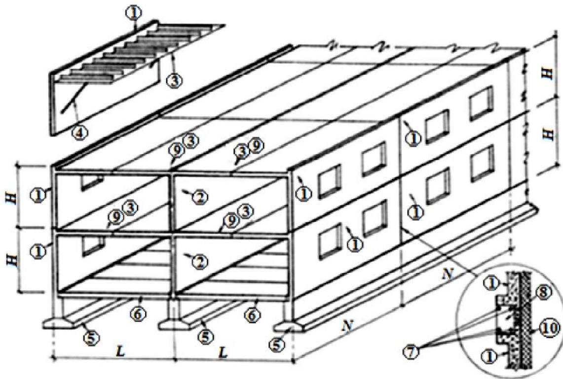
**Fig. 7.** Construction scheme for a building using spatial structures.
