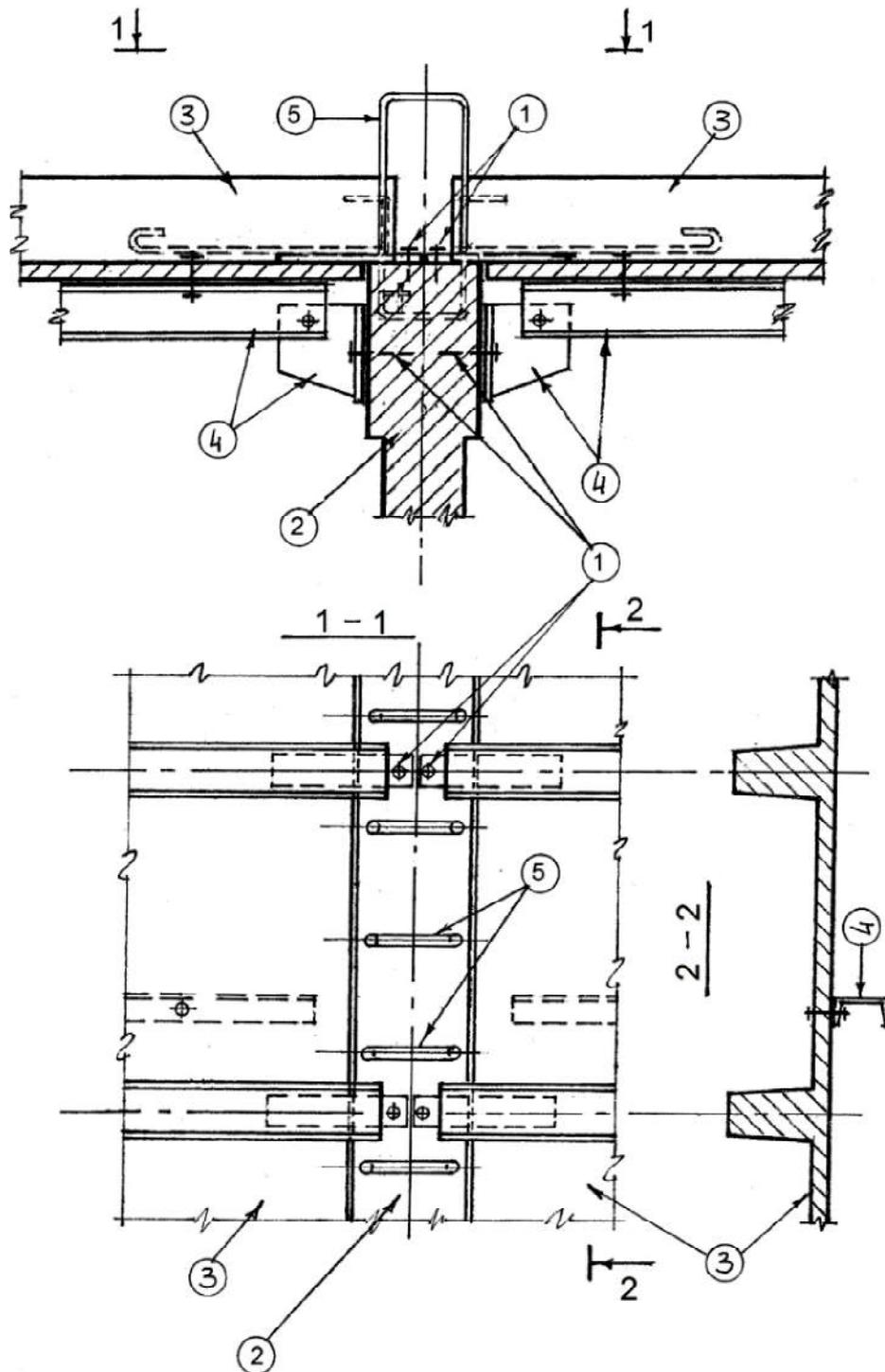
**Fig. 4.** Support scheme for a prefabricated precast concrete formwork (3) on an internal wall panel (2)
