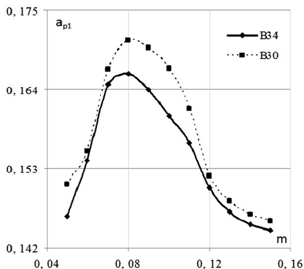
**Fig. 2.** Dependence of a coefficient of damping of an elastic longitudinal acoustic wave on the porosity of cement concrete
