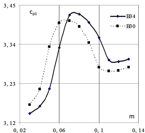
**Fig. 3.** Dependence of the propagation speed of an elastic acoustic wave on the porosity of cement concrete
