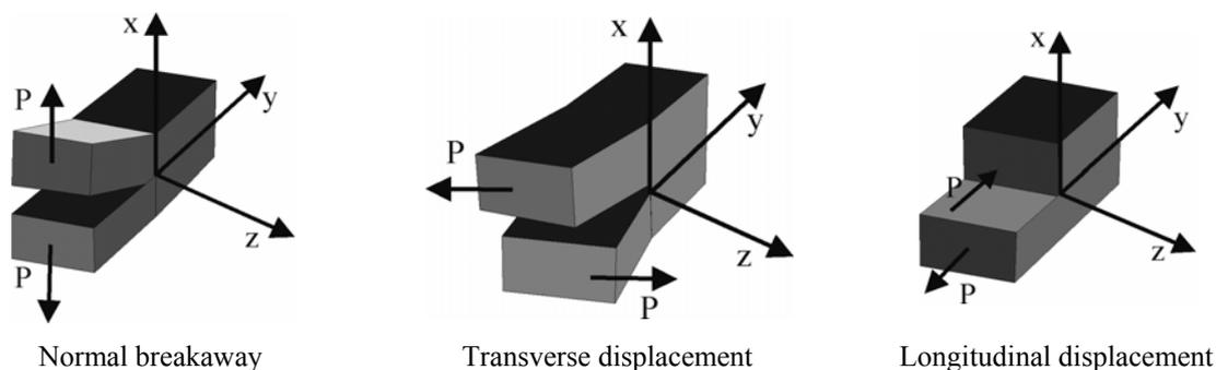
**Fig. 1.** Model of displacements of the crack edge during failure of solid bodies
