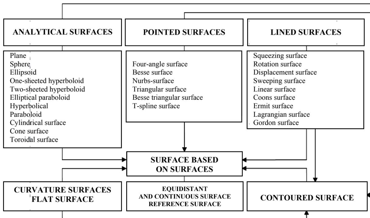
Fig. 2. Classification of surfaces in CAD and computer graphics
