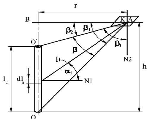
**Fig. 3.** Geometric designs for determining local angular coefficients of radiation of a linear source on an elementary area for their position in mutually perpendicular planes
