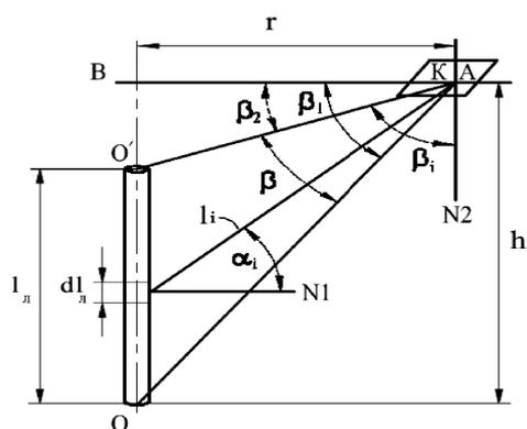
**Fig. 4.** Geometric designs for determining local angular coefficients of radiation for an elementary area on a horizontal plane at a random height
