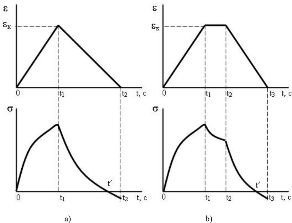
**Fig. 2.** Changes in the strains under the deformer for the triangular (a) and trapezoid (b) laws of the deformation of the material
