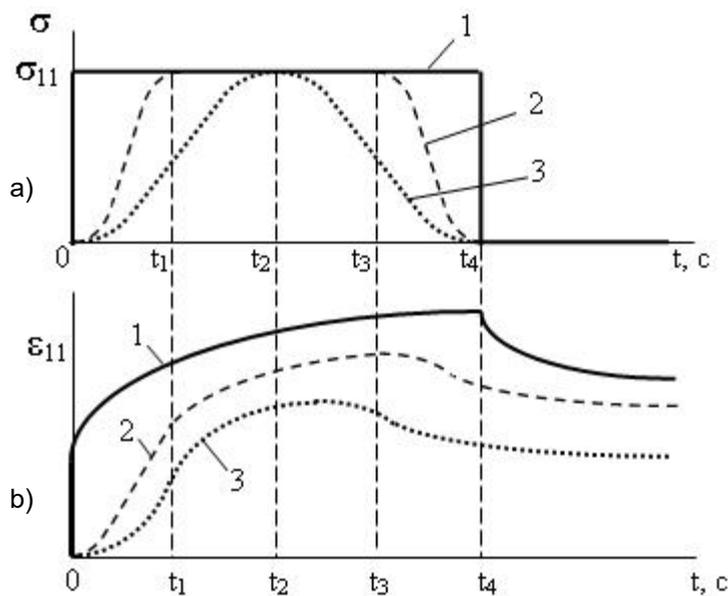
**Fig. 1.** Laws of loading a compacted layer:
