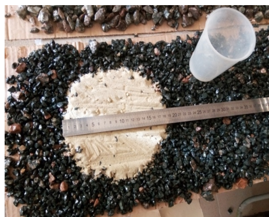
Fig. 11. Distribution of sand on the samples
