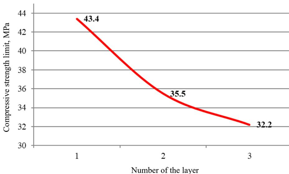
**Fig. 1.** Distribution of strength and speed of the ultrasound in the layers:
