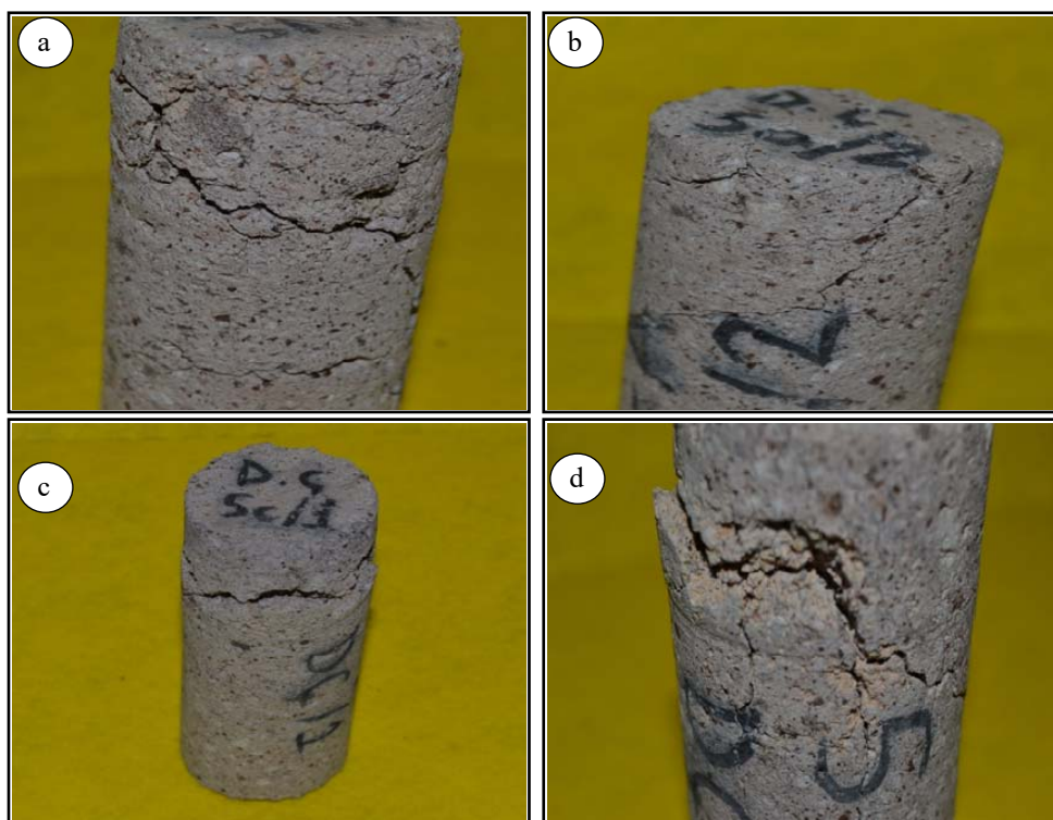
Fig. 5. Macro cracks as a result of F-T test (a) Sample 3 (b, c,d ), Sample 5
