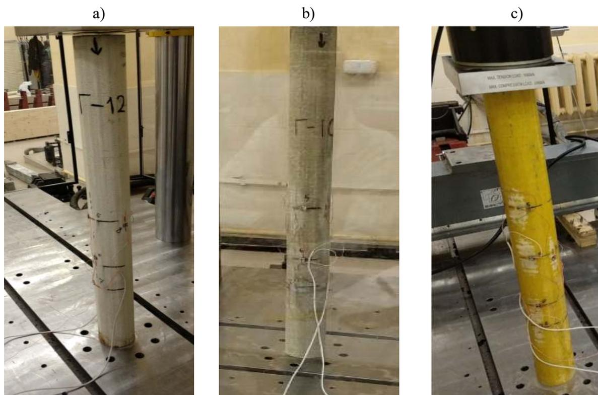
**Fig. 4.** Samples of concrete-filled hybrid poles 1 m long before compression test with fiberglass sheaths:
