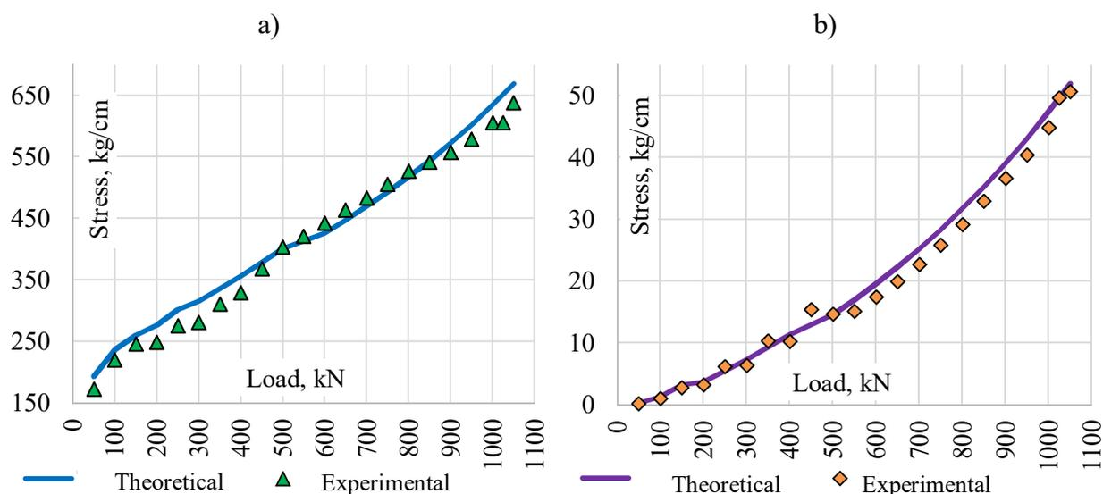
Fig. 8. Comparison of theoretical and experimental average stress values of the elements of hybrid racks for fiberglass shells of various grades filled with concrete: a) stresses of the concrete core in the longitudinal direction; b) transverse (radial) stresses
