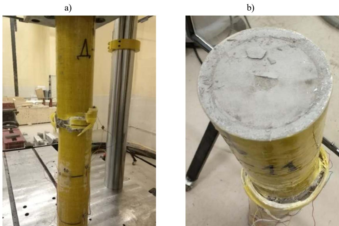
**Fig. 5.** Hybrid strut compression defects:
