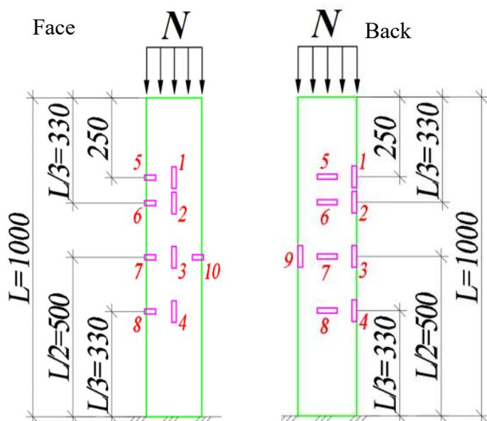
**Fig. 1.** Measurement of relative deformations: maps of places and directions installation of strain gauges on the samples
