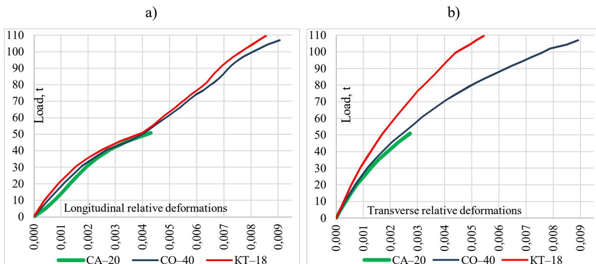
**Fig. 6.** Graphs of the increase in relative strains under compression for samples of hybrid racks 1 m long with shells made of diverse grades of fiberglass:
