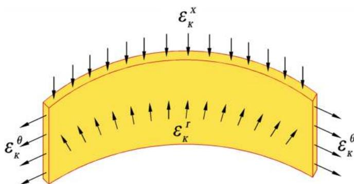
**Fig. 2.** Measurement of relative deformations: diagram to understanding directions relative deformations of the shell
