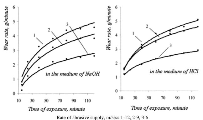
Fig. 2. Change in wear rate depending on time of exposure and type of aggressive medium at temperature of +5 °C
