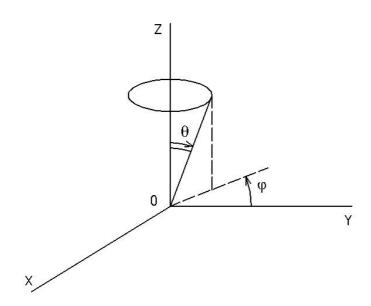
Fig. 1. Spherical coordinate system
