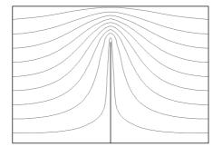
**Fig. 5.** Electric current lines in a premise with a partition and a horizontal one-way air flow
