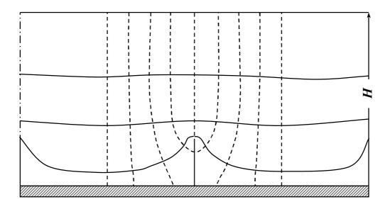
Fig. 3 shows isotherms and heat current paths inside the ribbed wall.
