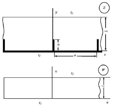
Fig. 4. Conformal mapping of the ribbed wall into a homogeneous one
