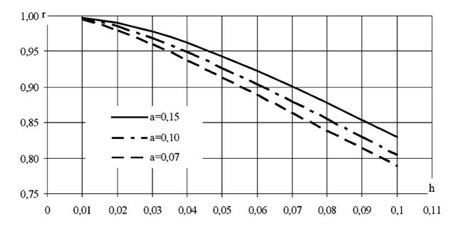
Fig. 5. Dependency of the coefficient of thermal and engineering integral r on the height of the rib h
