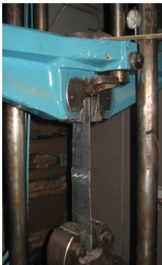
Fig. 8. Testing of the sample of the joint of the sheet metal samples on self-cutting screws during bend strengthening on a cutting machine
