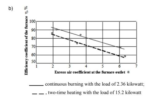
Fig. 1. Results of heating experiments in a gas heating furnace ( $Q_{cp}^u = 3.3 \text{ kilowatt}$ ) [2]:
