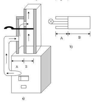
Fig. 2. Ventilation of the firebox of a gas heating furnace:a) general view of the furnace;b) valve
