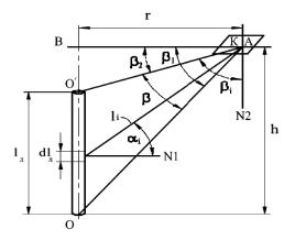
Fig. 3. Geometric designs for determining local angular coefficients of radiaiton of a linear source on an elementary area for their position in mutually perpendicular planes
