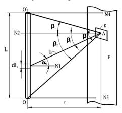
Fig. 1. Geometric designs for determining local angular coefficients of radiation of a linear source on an elementary area for its position in mutually parallel planes
