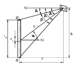
**Fig. 2**. Geometric designs for determining local angular coefficients of radiation for an elementary area on a vertical plane at a random height
