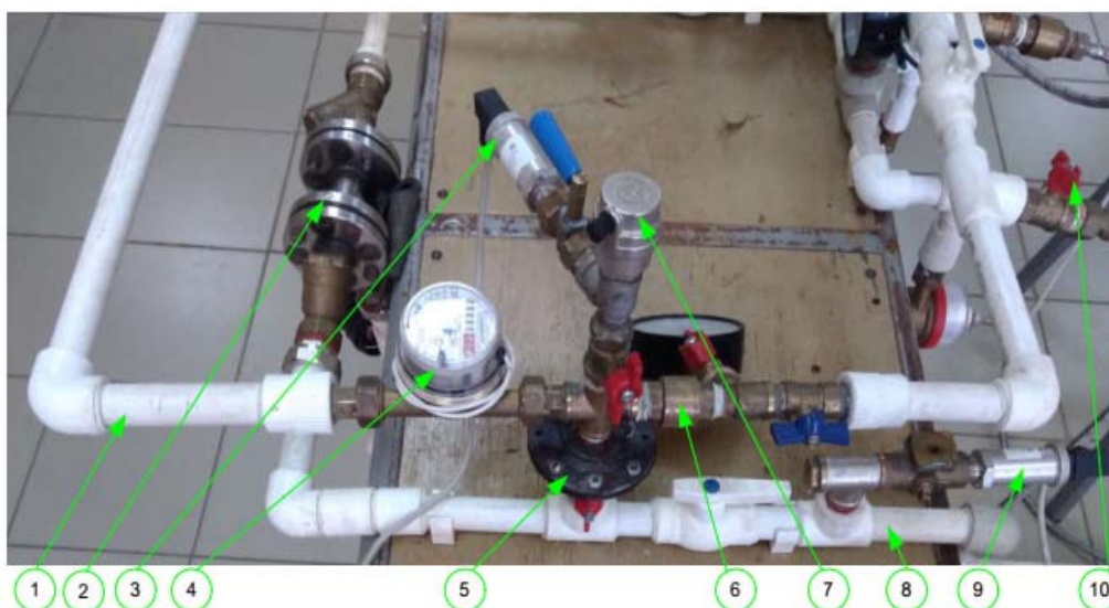
Fig. 3. Fragment of the scheme of the experimental setup for organizing impulse and pulsing circulation of liquids in the isolated contours:
