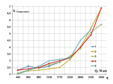
Fig. 8. Dependence of the number of the wells on the consumed energy of the heat pump with the transformation coefficient of no less than 2
