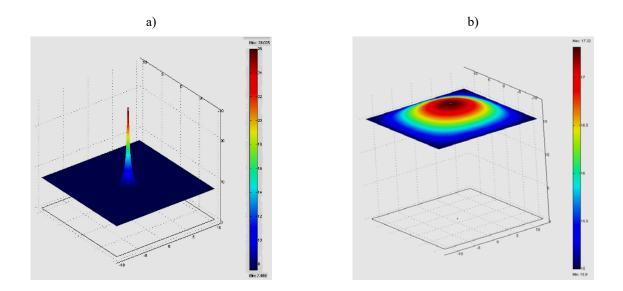
**Fig. 3.** Change in the temperature field: a) active load during 6 months; b) downtime mode of the heat pump
