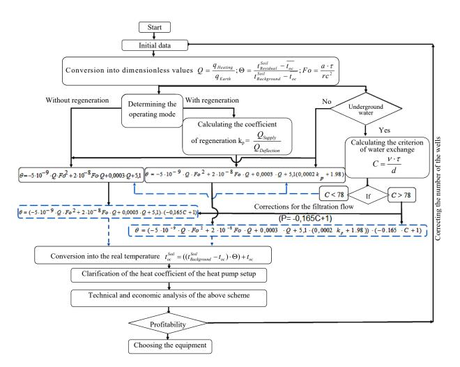
Fig. 9. Block scheme of the technical and economic parameters of the optimization of the composite systems of heat supply and air conditioning using a low-potential geothermal energy
