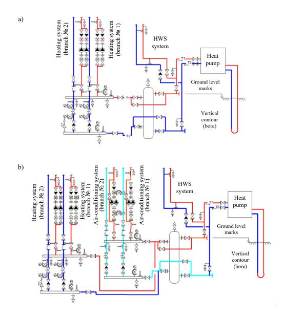
**Fig. 1.** Principal scheme: a) heat supply; b) heat supply – conditioning
