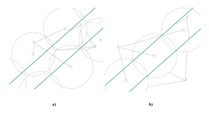
Fig. 1. Location of ECP facilities prior and following the reconstruction on parallel gas pipelines:a) prior to the reconstruction of the ECP; b) following the reconstruction of the ECP;1 are cathodic protection stations, 2 is a protective potential surfacing, 3 is an underground gas pipeline
