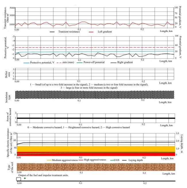
Fig. 3. Corrosion map of the pipeline
